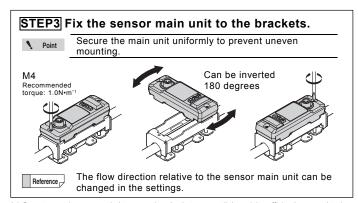
$^{\star}1\,$  Do not exceed recommended torque rating. Apply torque until the unit is sufficiently secured to the pipe. If you are mounting to thin-walled metal pipes or brittle resin pipes, contact KEYENCE for detail as damage may occur to the pipe even under the recommended torque rating.
