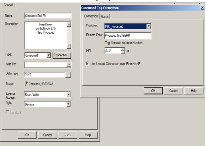
8. Check the tag Consumer type and ensure that the value is 0 before download the Producer Controller project
