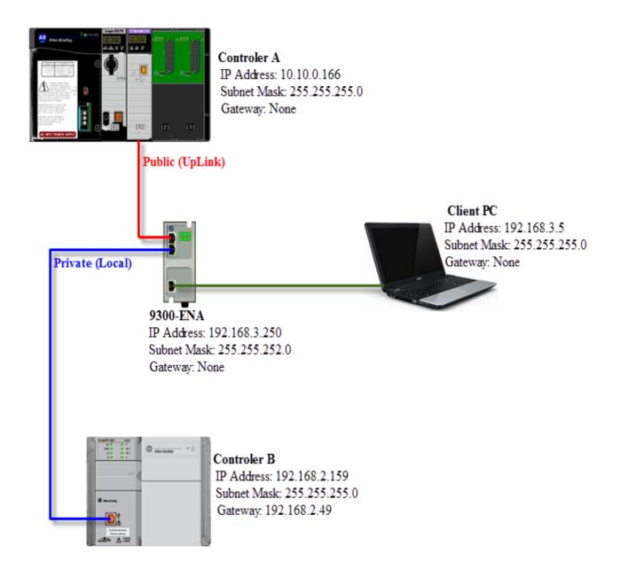
Note: Any changes on the 1783-NATR require a power cycle/module reset to take effect
