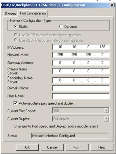
IP address of the ControlLogix controller
