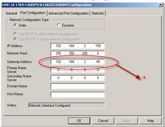
IP address of the CompactLogix
