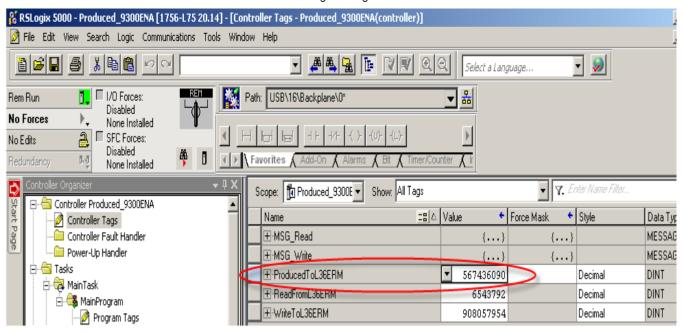
10. Check the tag Consumer type and ensure that the value 567436090 is there after downloading the Producer Controller project
